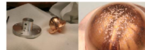
Copper button after 28 MV/m & 3 T
