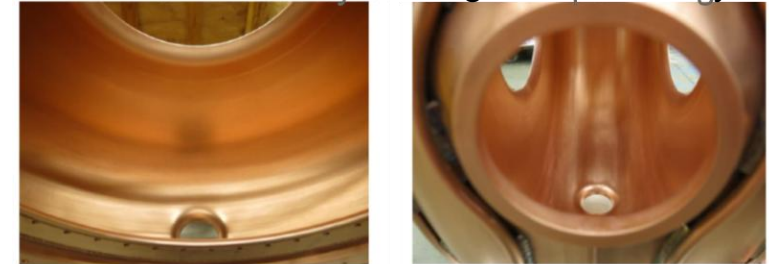
Mirro-like surface finishing in MICE cavity
