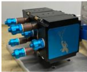
2-layer 3x3-crystal Crilin prototype
