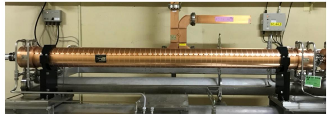
Bench test of S-band structure at KEK
